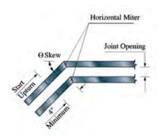
Typical Horizontal Miter Detail
